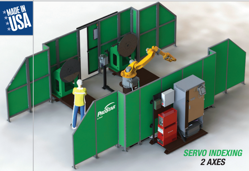
2 stations, single-axis positioners on opposite sides of the robot.
