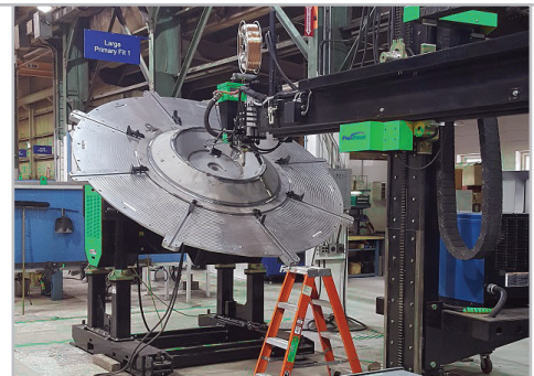
Fully integrated with manipulators or robotic welding
