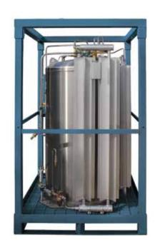
Portable, High-Performance PORTAFLEX™ 450 ZX VHP Microbulk Storage System Designed and built for high-pressure and high-flow applications, Linde's PORTAFLEX<sup>TM</sup> 450 ZX VHP microbulk storage system provides flexible portability to quickly respond to demanding industrial gas applications. Easily transported, the system is rated at flow rates of up to 2000 SCFH while sustaining 420-450 psig.
