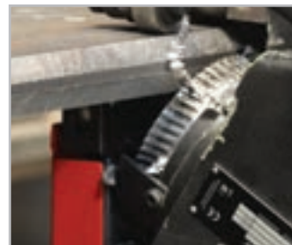
180° inversion allows for quick and easy creation of double-sided bevels
