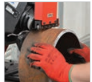
Self-feeding for consistent bevel geometry from end-to-end.
