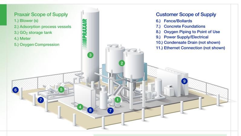
For customers needing up to 62 tons per day of oxygen, the ideal supply is Praxair's V40 S-XL. The V40 S-XL is a vacuum pressure swing adsorption (VPSA) plant that consists of a feed blower, sieve beds, vacuum blowers, surge tank and silencers. The system is designed and shipped on two skids - allowing very rapid field installation and minimum disruption to your site. Product delivery pressure is tailored to each customer's unique requirement.
