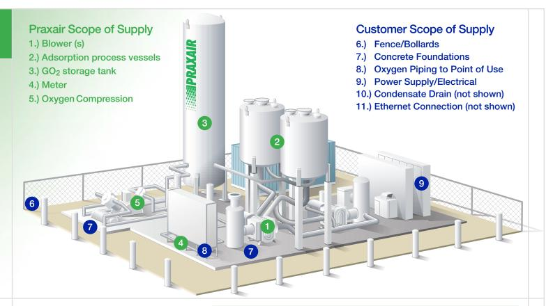
For customers needing up to 218 tons per day of oxygen, the ideal supply is Praxair's V120 XL-XXL. The V120 XL-XXL is a vacuum pressure swing adsorption (VPSA) plant that consists of a feed blower, sieve beds, vacuum blowers, surge tank and silencers. The system is designed and shipped on five skids - allowing very rapid field installation and minimum disruption to your site. Product delivery pressure is tailored to each customer's unique requirement.
