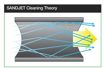
The first cleaning run is performed by loading a calculated amount of cleaning material, usually a few hundred pounds, into the cleaning material hopper. An appropriate nitrogen flow rate is established throughout the system and cleaning material is fed into the injection head where it fluidizes with
