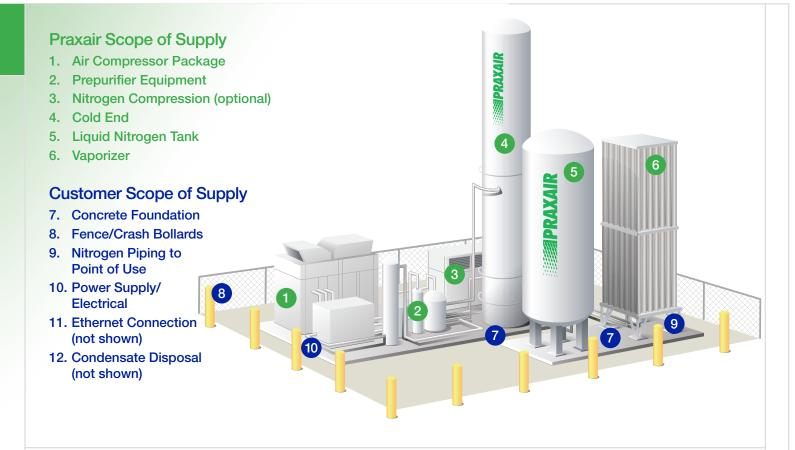
For customers needing up to 56,100 cfh-ntp of nitrogen, the ideal supply is Praxair's N40 XL. The N40 XL is a cryogenic nitrogen plant that consists of a Warm End which includes the air compressor package and prepurifier equipment, and a Cold End which includes the distillation column, primary heat exchanger, and main condenser. The N40 XL uses liquid assist for the refrigeration requirement of the plant. The system also comes with a liquid nitrogen **Backup** System for ultimate reliability.
