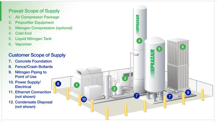
For customers needing up to 61,900 cfh-ntp of nitrogen, the ideal supply is Praxair's N50. The N50 is a cryogenic nitrogen plant that consists of a **Warm End** which includes the air compressor package and prepurifier equipment, and a **Cold End** which includes the distillation column, primary heat exchanger, and main condenser. The N50 uses liquid assist for the refrigeration requirement of the plant. The system also comes with a liquid nitrogen **Backup System** for ultimate reliability.
