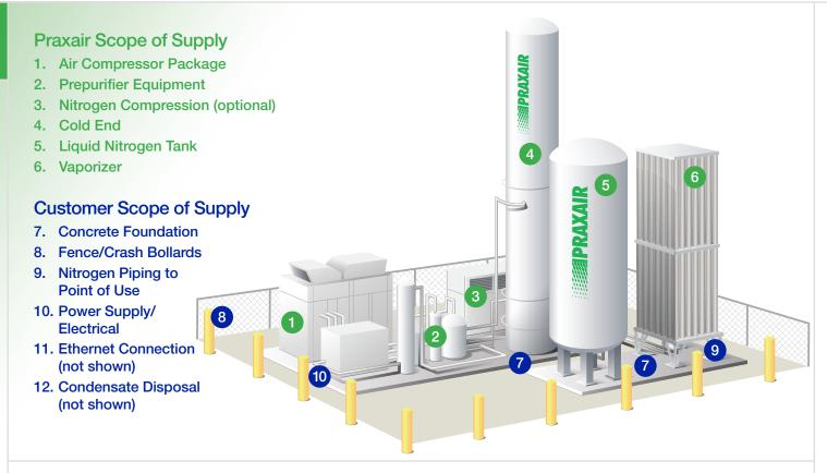
For customers needing up to 211,800 cfh-ntp of nitrogen, the ideal supply is Praxair's N180. The N180 is a cryogenic nitrogen plant that consists of a Warm End which includes the air compressor package, electrical equipment and switching valves, and a Cold End which includes the distillation column, primary heat exchanger, and main condenser. The system also comes with a liquid nitrogen Backup System for ultimate reliability.
