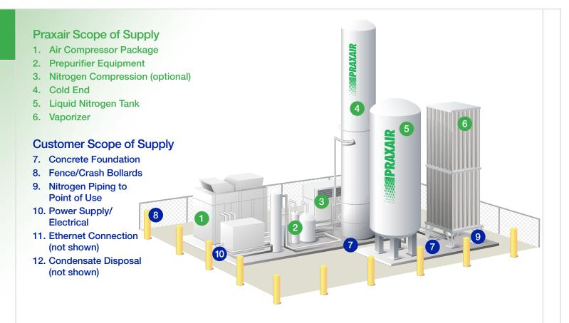
For customers needing up to 25,900 cfh-ntp of nitrogen, the ideal supply is Praxair's N15. The N15 is a cryogenic nitrogen plant that consists of a **Warm End** which includes the air compressor package and prepurifier equipment, and a **Cold End** which includes the distillation column, primary heat exchanger, and main condenser. The N15 uses liquid assist for the refrigeration requirement of the plant. The system also comes with a liquid nitrogen **Backup System** for ultimate reliability.
